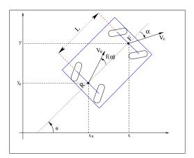
Figure 1: Model of the Bi-steerable car.
