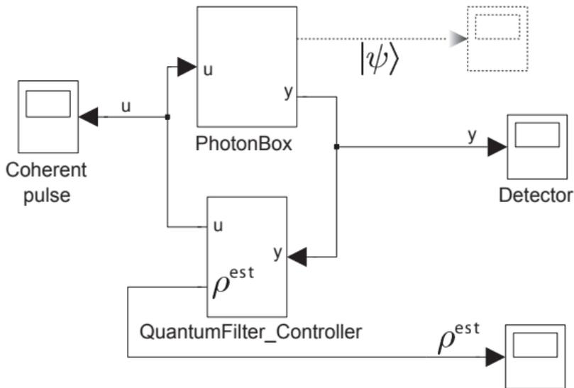
The **state estimation**  $\rho_k^{\text{est}}$  used in the feedback law takes into account, measurement imperfections, delays and cavity decoherence:
