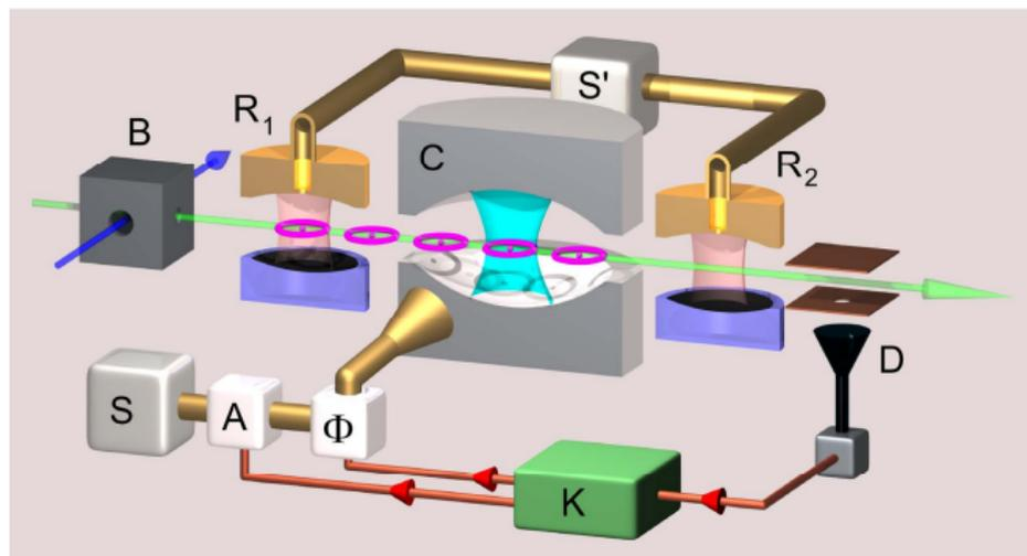
Stabilization by a **measurement-based feedback** of photon-number states (sampling time  $80 \mu\text{s}$ )
