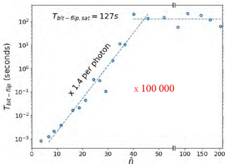
FIG. 4. Exponential suppression of bit flips. The bit-flip time (y-axis, log-scale) is measured (open circles) as a function of cat-size (x-axis). The bit-flip time increases exponentially, multiplying by 1.4 per photon (solid line) before saturating at approximately 127 s (horizontal dashed line).
