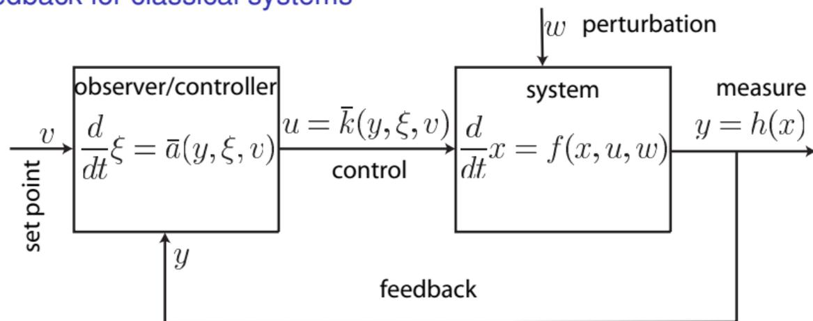
**Proportional Integral Derivative (PID)** for  $\frac{d^2}{dt^2}y = -\omega^2 y + u + w$  with the set point  $v = y_{sp}$
