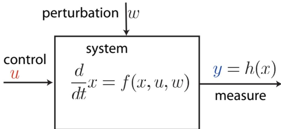
For the **harmonic oscillator** of pulsation  $\omega$  with **measured position**  $y$ , **controlled by the force**  $u$  and subject to an additional unknown force  $w$ .
