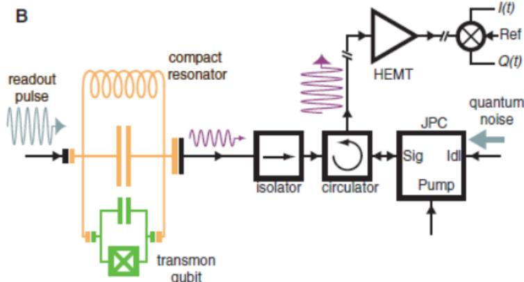
**Superconducting qubit** dispersively coupled to a cavity traversed by a microwave signal (input/output theory). The back-action on the qubit state of a single measurement of both output field quadratures  $I_t$  and  $Q_t$  is described by a simple SME for the qubit density operator.
