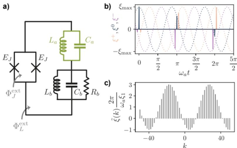
High impedance  $\sqrt{L_a/C_a}$  and low pulsation  $1/\sqrt{L_a C_a}$  for storage mode  $\hat{a}$ .
