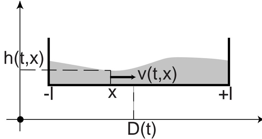
$$\frac{\partial h}{\partial t} + \frac{\partial(hv)}{\partial x} = 0, \quad \frac{\partial v}{\partial t} + \ddot{D} + v \frac{\partial v}{\partial x} = -g \frac{\partial h}{\partial x}$$
