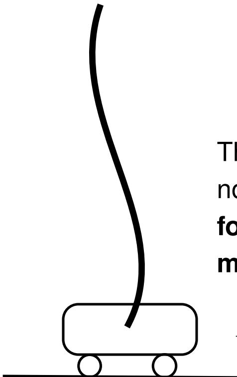
$$\frac{\partial}{\partial z} \left( gz \frac{\partial X}{\partial z} \right) + \frac{\partial^2 X}{\partial t^2} = 0$$
