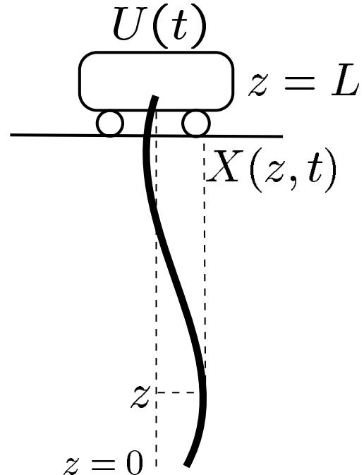
$$\frac{\partial^2 X}{\partial t^2} = \frac{\partial}{\partial z} \left( g z \frac{\partial X}{\partial z} \right)$$
