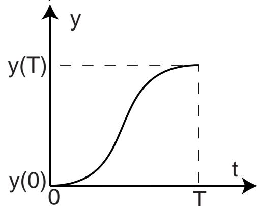
$$\begin{aligned}\dot{y} &= \ddot{y} = y^{(3)} = y^{(4)} = 0 \text{ for } t = 0 \\ \dot{y} &= \ddot{y} = y^{(3)} = y^{(4)} = 0 \text{ for } t = T\end{aligned}$$
