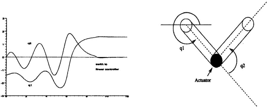
Figure 1: Swingup and Balance of The Acrobot
