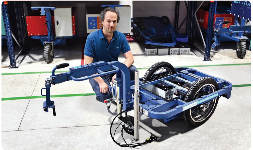
Nicolas Petit next to a K-Ryole 5, a smart electric trailer allowing bikers to effortlessly transport up to 350 kg, for which he designed the embedded control algorithms. As of August 2020, independent delivery companies operate more than 100 of these trailers daily in Paris.
