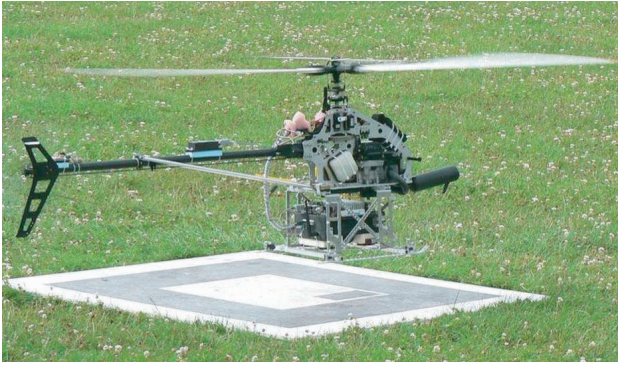
Fig. 1. “Goliath”, our helicopter equipped with low-cost sensors in hover flight.
