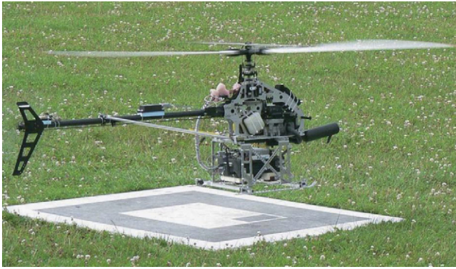
Fig. 1. "Goliath", the helicopter equipped with low-cost sensors in hover flight.
