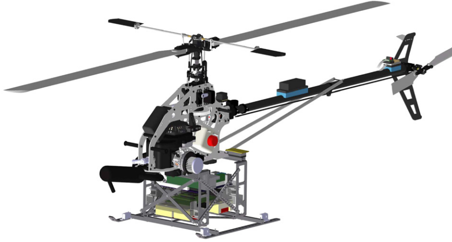
Fig. 8. Three dimensional view of the CATIA® model of the helicopter. Six hundred and eighty parts are modeled and kinematically linked together. The obtained model is pictured in Fig. 8. Payload, landing-gear, sensors, electronic devices, Li-Po batteries, and numerous add-ons are modeled to obtain accurate estimates of inertia matrix and position of the center of gravity.
